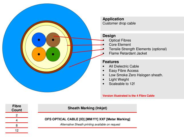
Cable Diameter (calc.): Cable Weight (calc.): 3.5 mm 8.5 kg/km
